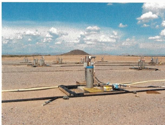
Figure 6. a) In-situ leach well field (established during a production test by BHP Copper in 1997-1998) at Florence, Arizona. b) Conventional open pit operation at ASARCO's Mission mine near Tucson, Arizona
